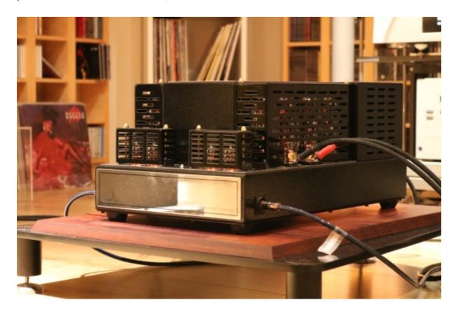
The JL5 even uses the same driver tube technology as THE STATEMENT amplifier. This driver is specifically optimized for the high current KT120 tube. The new JL5 is said to deliver the "drive anything" sound of its bigger brothers while being fully competitive with the older 6550 version of the more expensive JL2.
