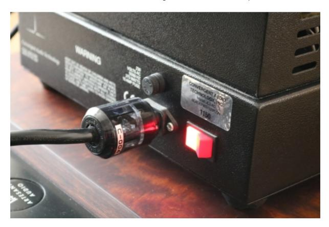
Power amplifiers do not get any simpler to connect than the JL5. There's nothing on the rear end but the power inlet and a big power switch
