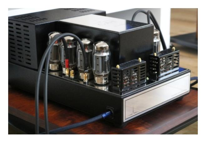
JL5 with the Tube-Protector cages removed. This is necessary when using banana connectors.
